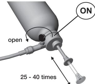
The air pressure in the fuel bottle is crucial to the heat of the stove. When preparing food, you may have to do some more pumping in order to maintain maximum heat. However, if you pump up too high a pressure the fuel flow will be too great resulting in a yellow flame.
