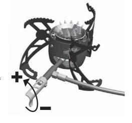
10-15 seconds, the burner is not hot enough and you have to preheat the stove for a little longer. In this case, close the control valve one more time, wait until the flames are almost out and then open the control valve again.
